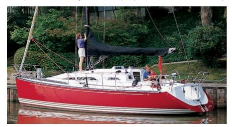
The hull is easily driven, and well balanced. Jackett computer-modeled over 200 hull forms before he was satisfied he'd found the hull shape with the right distribution of fore-and-aft volume—a critical factor in producing a design that's not only a strong performer, but can also support a full-fledged interior.
